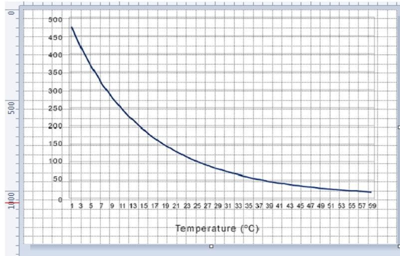
Figure 2 - Illustrates the resistance of the thermistor as a function of the temperature
