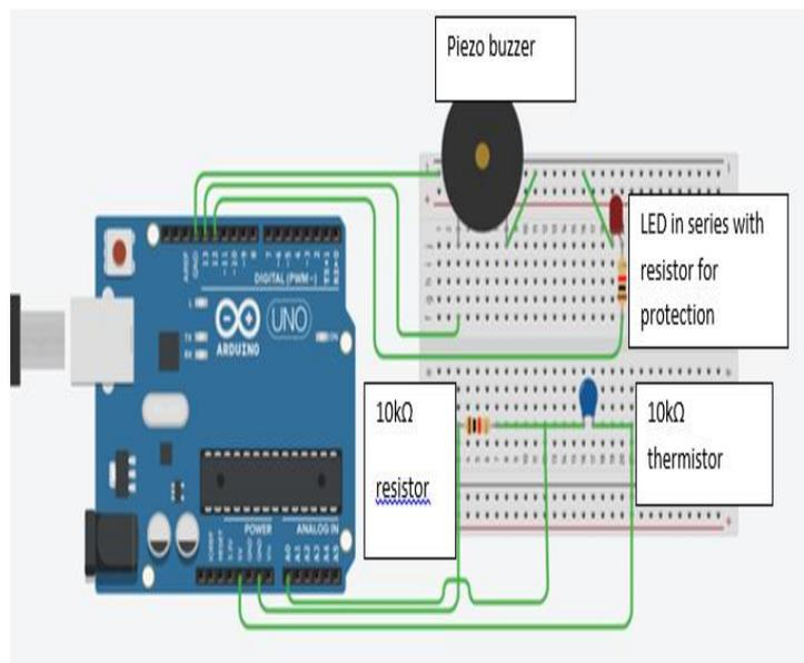
Figure 4 – Experimental setup of designed fire detector
