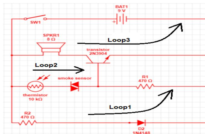
Figure 3 – Basic circuit diagram of fire detector with series connected thermistor and smoke sensor
