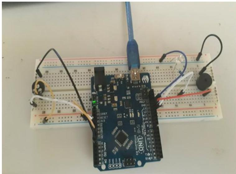
Figure 5 – Model of Arduino-integrated fire detector
